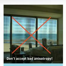
**Anisotropy** is currently the hottest topic in glass processing. Thanks to a new slot nozzle design in the chiller, stress level differences, and thus anisotropy, can be radically reduced.
